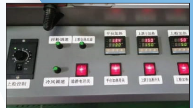
Temperature controls of the Hot Melt Adhesive Powder Spraying Machine.
